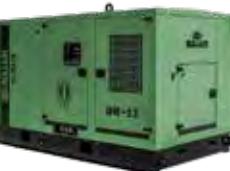
THE SULLAIR DR-13 Class 0 Oil Free Air 428–785 cfm at 100–150 psig — 12.2–21.9 m³/min at 8.5 bar
